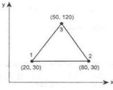
14 a. For the axisymmetric elements shown in Fig, determine the element stresses. Let E = 210GPa and  $\gamma = 0.25$ . The co-ordinates (in millimeters) are in shown Fig. The nodal displacements are:  $u_1 = 0.05$  mm;  $w_1 = 0.03$ mm  $u_2 = 0.02$  mm;  $w_2 = 0.02$ mm  $u_3 = 0$  mm;  $w_3 = 0$  mm
